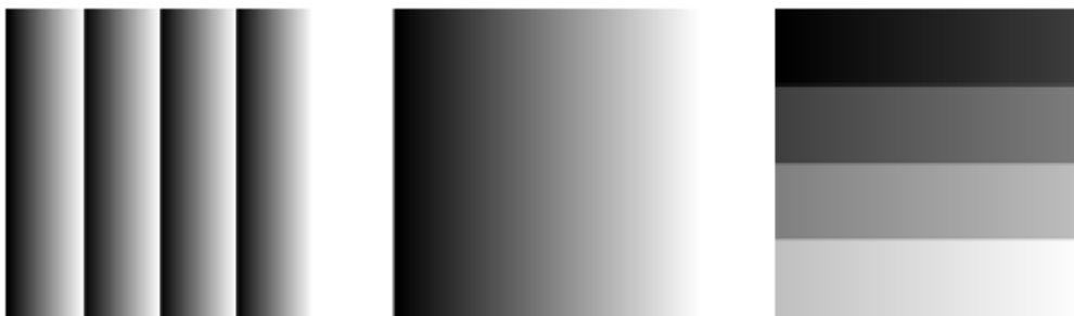
Figure 31: Ramp test images: 8 bit output (left), 10 bit output (middle), 12 (right)
