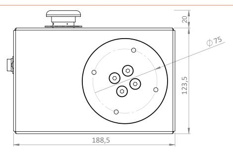
Figure 4: Dimensions - Top View
