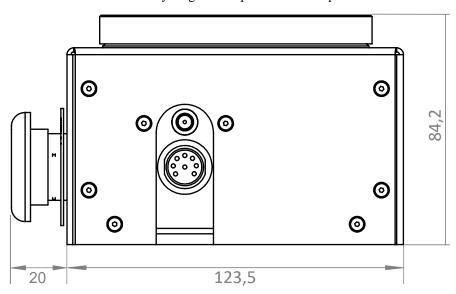
Figure 3: Dimensions - Front View
